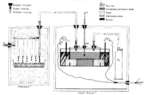
Fig. 1. Electrophoretic tank in partial section. Top of the tank and cooling system not shown (see fig. 2). All measurements in mm. Legend: A = large agar blocks, B = buffer compartments, C = agar connection slit, P = petroleum ether compartment, S = slide with agar film below, in contact with large agar blocks, (+) and (-) = electrodes; stippled areas represent agar.
